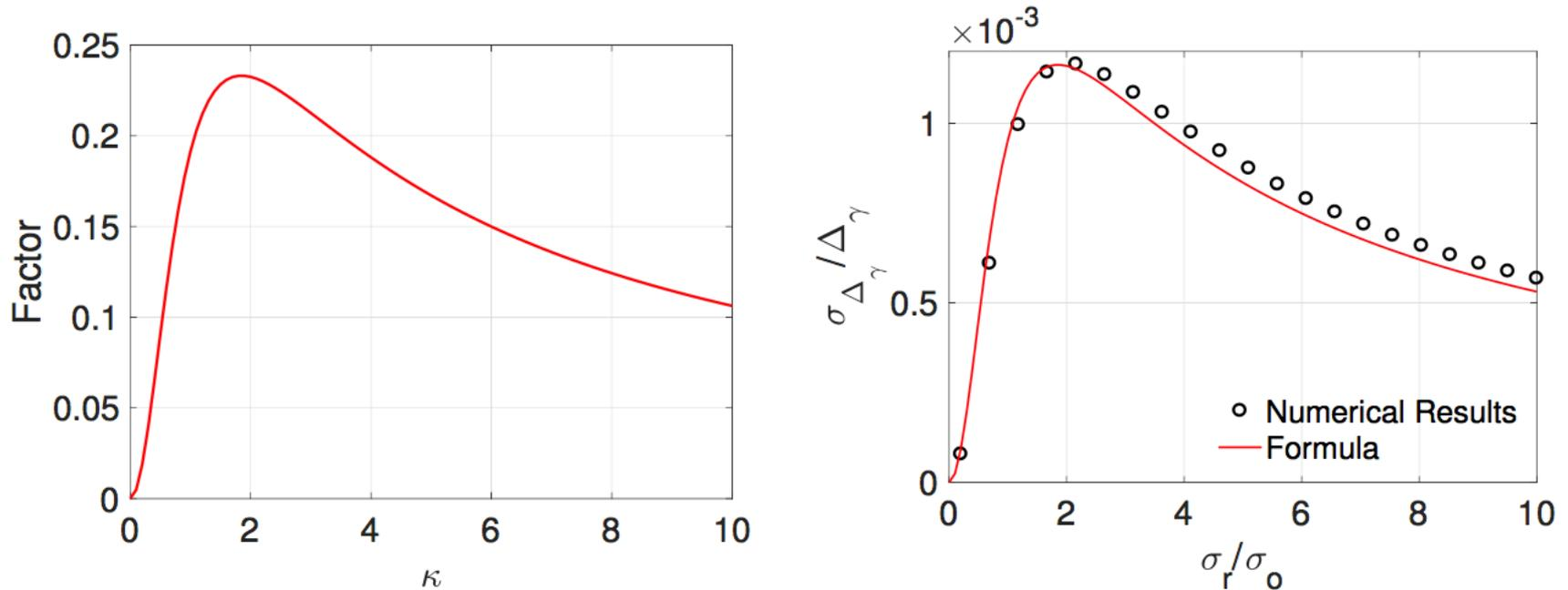
Figure 1: Left: The dependence of the factor on  $\kappa$ . Right: the comparison of the slice energy spread from numerical calculations (black circles) and the formula (red line). Parameters:  $E_i = 8$  GeV,  $E_{z0} = 2$ ,  $\Delta E_z = 0.01$  and the acceleration distance is  $L = 8000$ . Because the spot size of the beam decreases as the energy grows, there is small difference between the numerical results and the formula.
