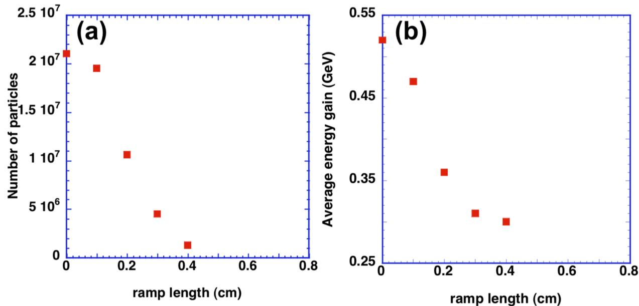
Figure 38: The number of positrons in the beam load (a), the average energy (red square) (b) of the beam load versus the ramp length at a propagation distance of 12cm.
