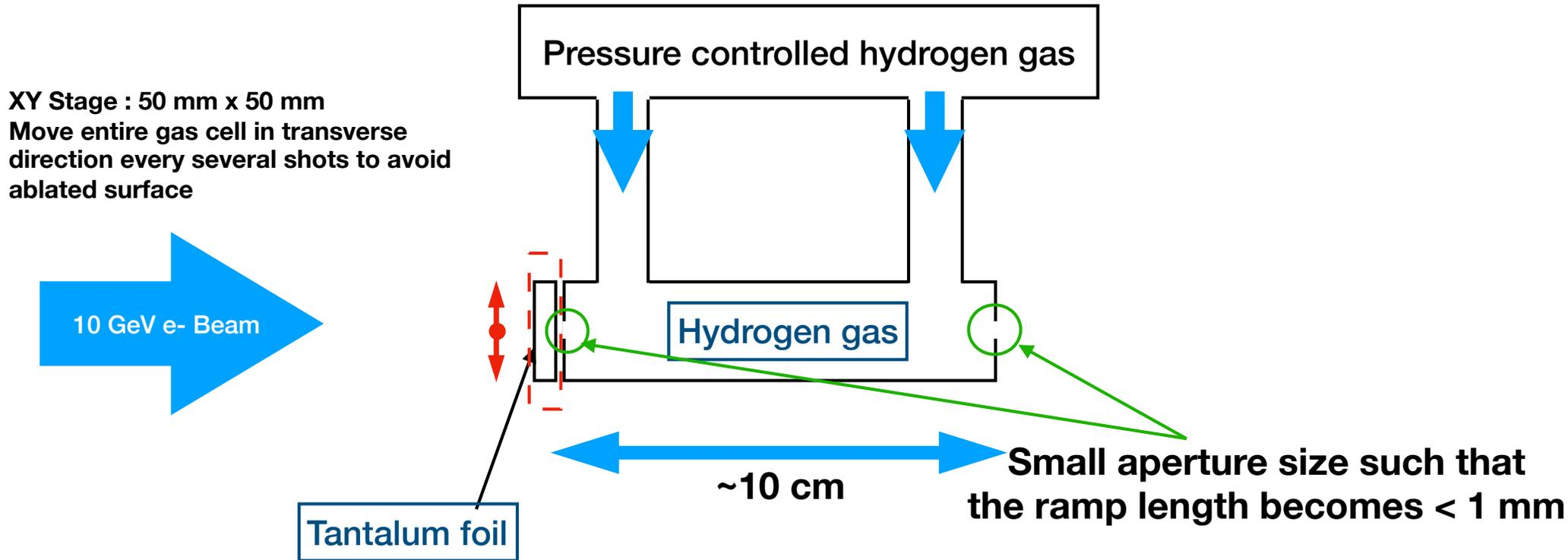
Allow gas leak at the each end of gas cell
